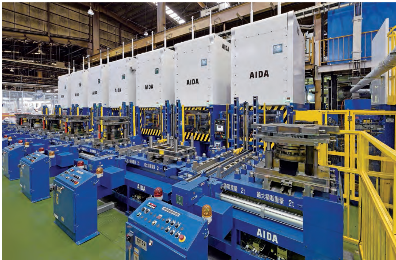
A compact high speed servo tandem line of seven DSF-N1-2000A equipped with NCAH-III(S) transfer robot system
